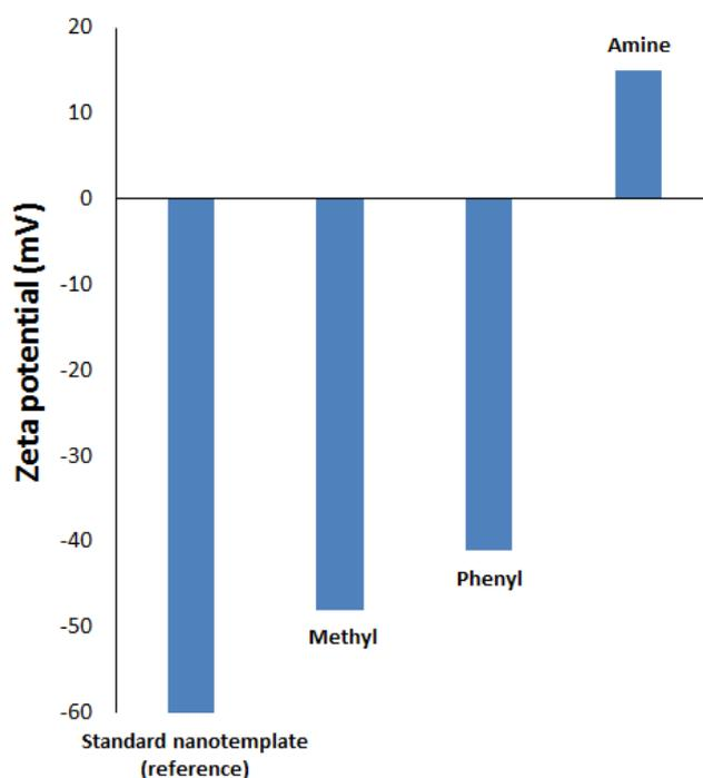
Figure 9. Zeta potential of the nanoparticles obtained from Method B and functionalised nanoparticles with methyl, phenyl and amine functionalities.
