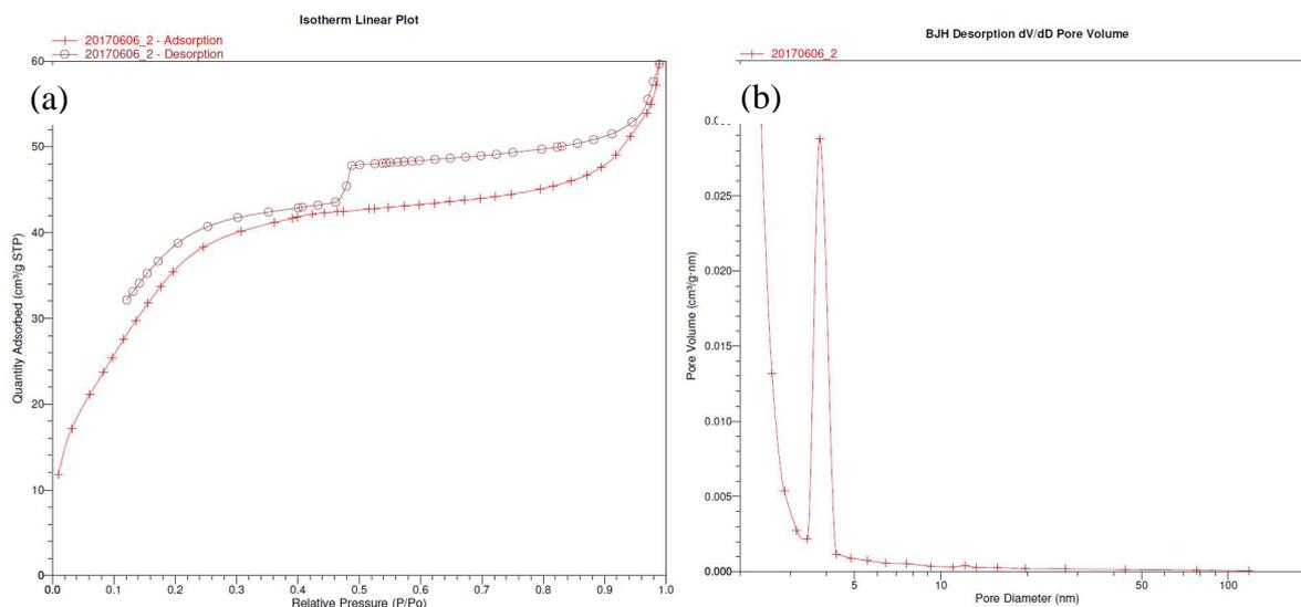
Figure 6. (a) Nitrogen adsorption and desorption isotherm for nanotemplate obtained with the Stöber route and (b) Pore size distribution of the same sample determined by BJH.
