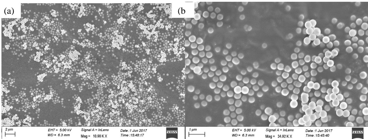
Figure 4 (a) SEM image of nanoparticles obtained with the Stöber route and (b) high resolution SEM image of the same nanoparticles.
