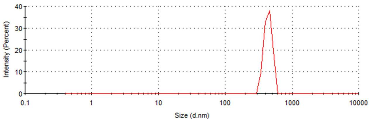
Figure 5. DLS data showing the hydrodynamic diameter of nanoparticles obtained with the Stöber route.
