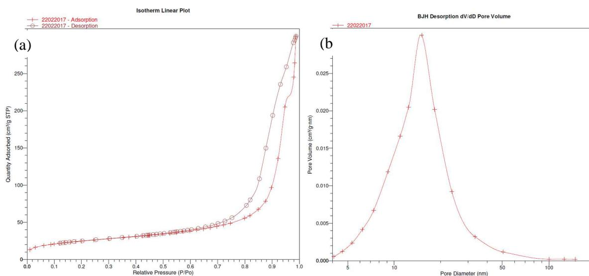
Figure 2. (a) Nitrogen adsorption and desorption isotherm for 3D nanotemplate obtained with Method A and (b) Pore size distribution of the same sample.
