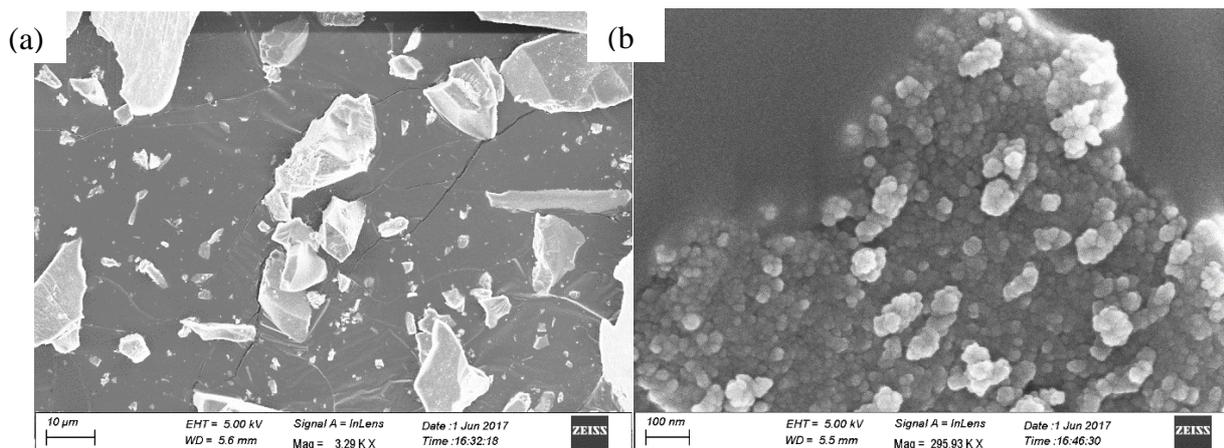
Figure 1. (a) SEM image of 3D nanotemplate obtained with Method A and, (b) higher resolution image of the nanotemplates synthesized.
