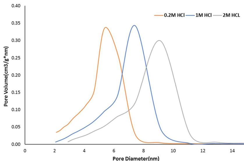
Figure 3. The effect of hydrochloric acid concentration on the pore size of the 3D Nanotemplates, obtaining pores of 5.5 nm, 7.3 nm and 9.4 nm (peak value).
