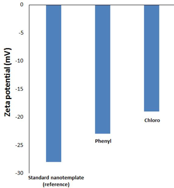
Figure 7. Zeta potential of standard 3D Nanotemplates and silanised nanotemplates with phenyl and chloro functionalities.
