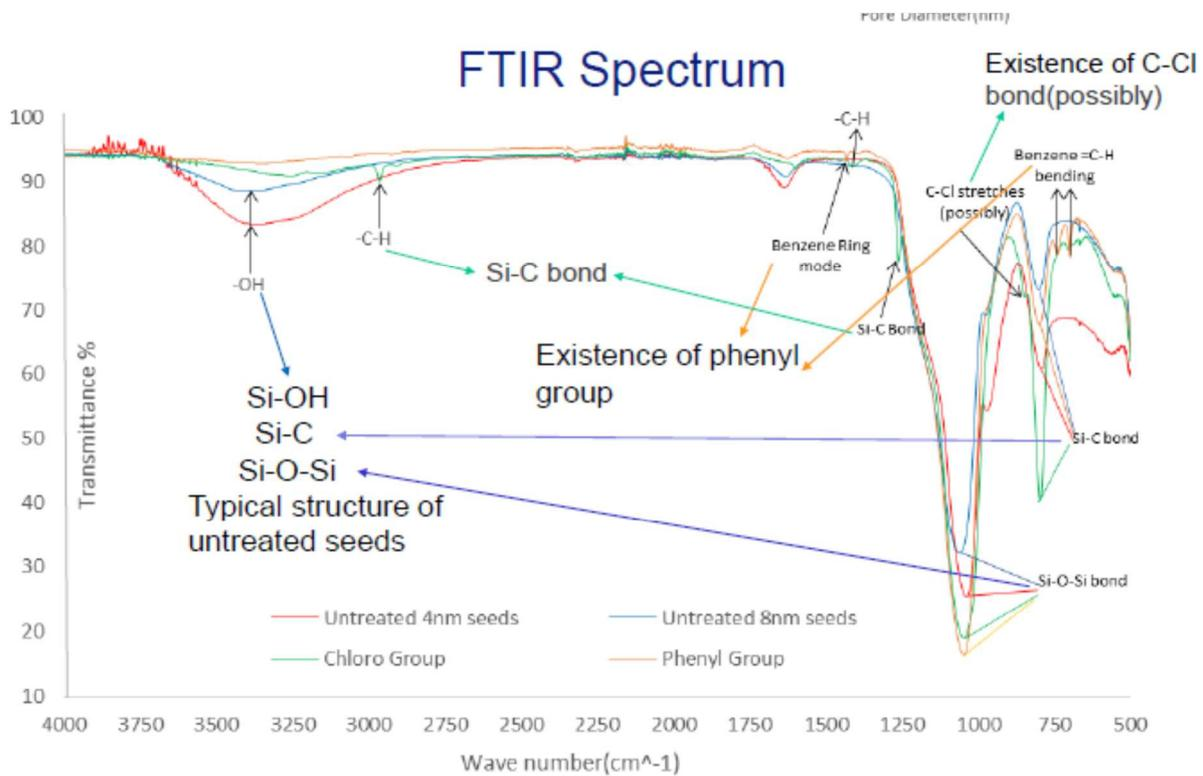
Figure 8. FTIR spectrum for non-functionalised and functionalised 3D Nanotemplates.
